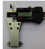
Thread inserts types 22 and 27 can overlap and measure pitch diameter on small diameter threads.
