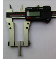
Thread inserts types 22 and 27 can overlap and measure pitch diameter on small diameter threads.
